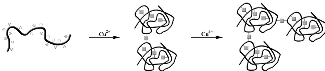
**Scheme 2**. Three-dimensional proposed structure model for poly(MVE-MA)-Cu<sup>2+</sup> binary complex. Filled square binding between COO<sup>-</sup> groups in Cu<sup>2+</sup> presence.
