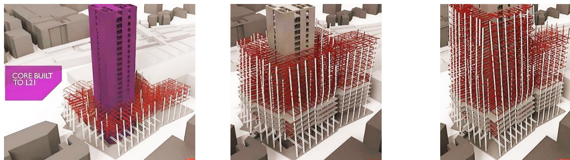
Figure 9. Core mass and continued construction of the structure (URL-6)
