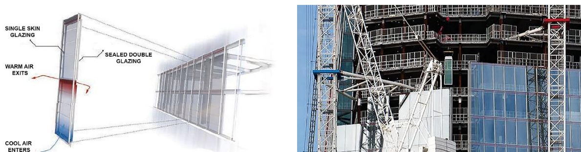
Figure 14. Glass module views of the facade (URL-17), (Cable, 2012)
